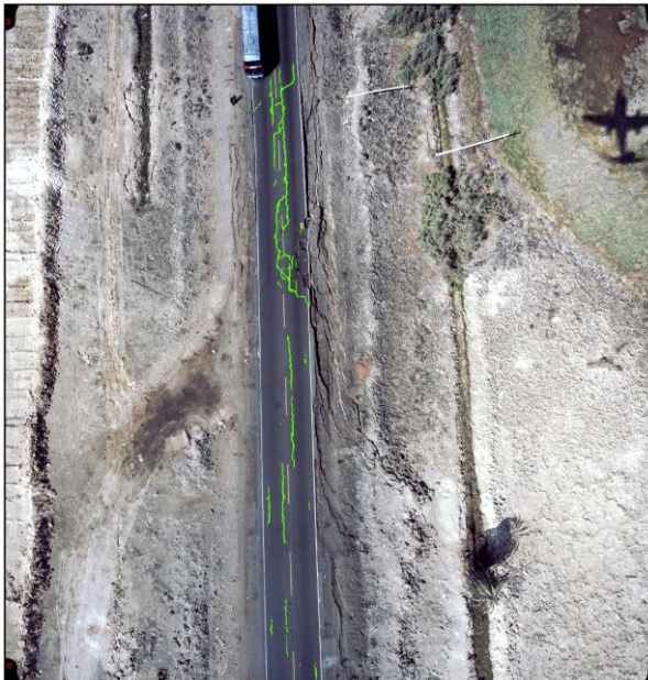
Fig. 8. Post-Earthquake Pavement Crack Detection Results.
