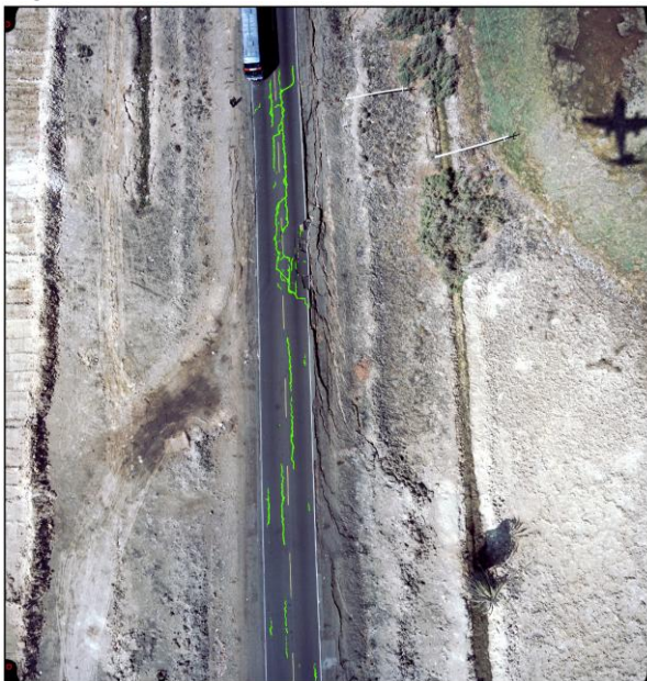
Fig. 8. Post-Earthquake Pavement Crack Detection Results.
