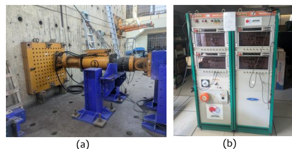
Fig. 1. The CISMID's Laboratory Actuator system: (a) Servo-hydraulic actuator, (b) Servo-controller.
