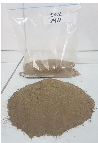
Fig. 3. Fine soil classified as elastic silt MH.
