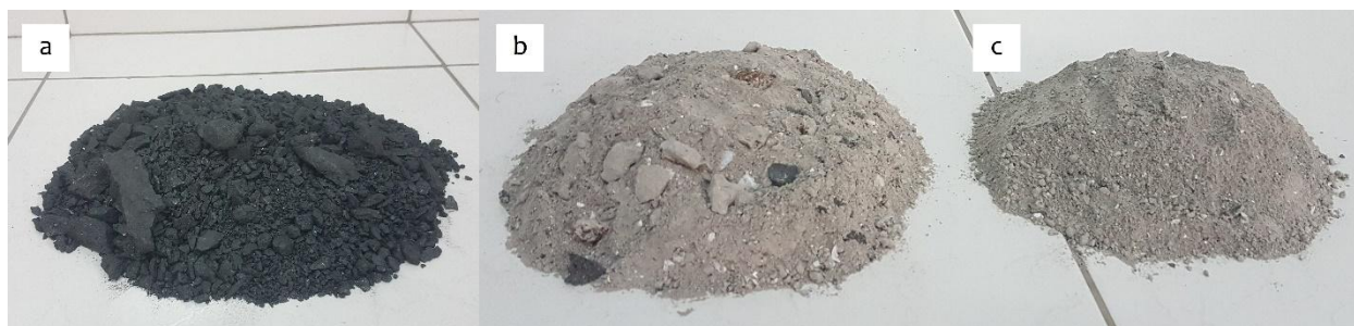
Fig. 4. a) Mineral coal used in combustion; b) Overall sample of bottom ash extracted from the kilns; c) Bottom ash sample sieved through No. 4 mesh for use in the tests.
