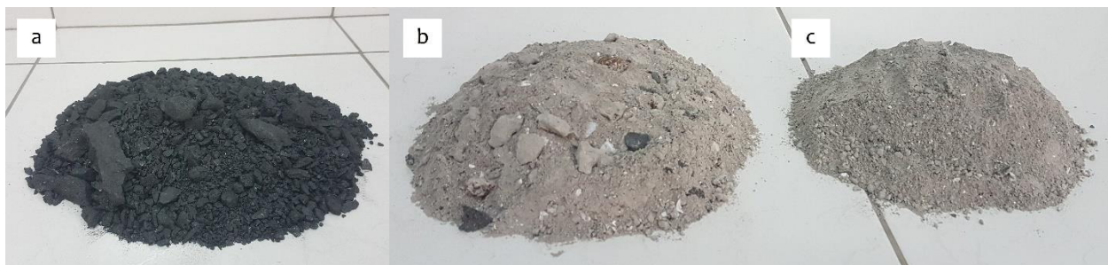
Fig. 4. a) Mineral coal used in combustion; b) Overall sample of bottom ash extracted from the kilns; c) Bottom ash sample sieved through No. 4 mesh for use in the tests.
